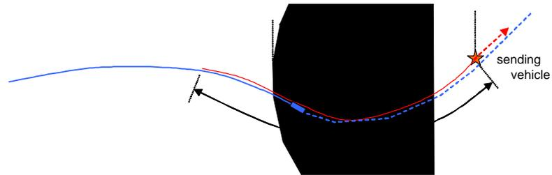
**Figure 5: Follower vehicle uses driven *and* predicted track (full and dotted blue lines)**
