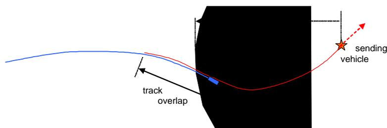
**Figure 4 : Following vehicle uses only driven track to detect match.**
