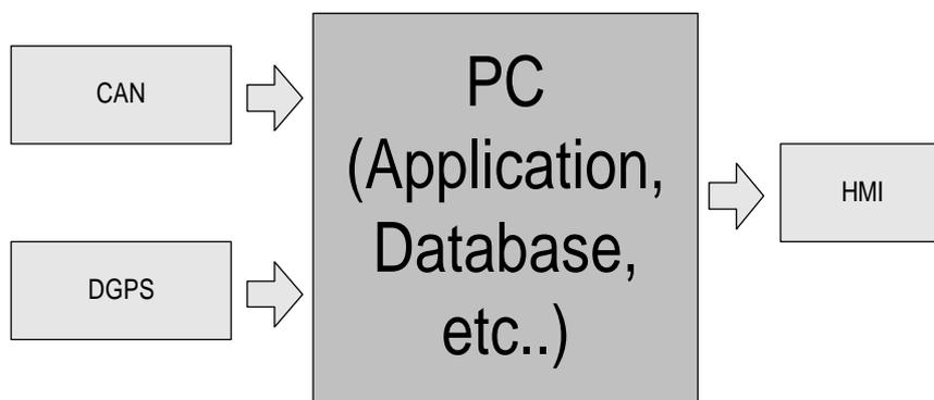
**Figure 2: BMW client hardware architecture.**
