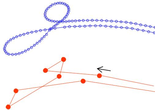
**Figure 6: Position trace (top) and cast trace points representing vehicle's driven path (bottom)**
