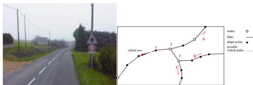
**Figure1: Any car mounted sensor (e.g. camera) provides information of the real world near the vehicle. An appropriate part of an enhanced digital map offers a wider 'view' on the surroundings for driver assistance applications.**
